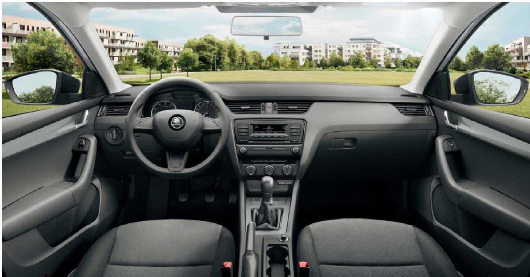
The Active version interior includes decorative elements, such as chrome door handles and black air-ventilation frames. The standard equipment covers electric front windows as well as electrically-adjustable heated external mirrors.
