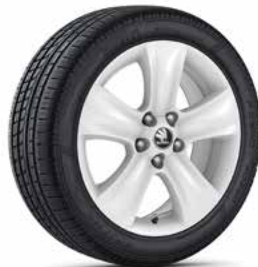
Dolomite light-alloy wheel 7,0J x 17" for 225/50 R17 tyres in white design (5L0 071 497N FM9)
