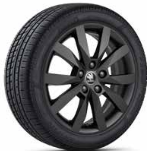
Crystal light-alloy wheel 6,0J x 17" for 205/50 R17 tyres in black metallic design, (5E0 071 497E FL8) suitable for snow chains
