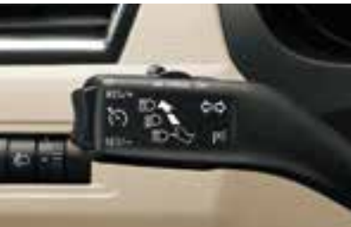
Cruise control for all engine versions for cars with on-board computer (5JB 054 690); for cars without on-board computer (5JB 054 690A)
