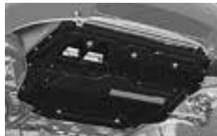
Protective engine cover for motor vehicles with petrol engines (5JA 071 608); for vehicles with diesel engines (5JA 071 608A)
