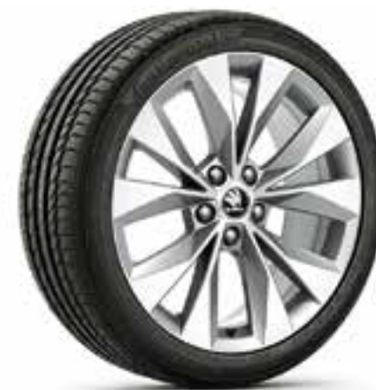
Cassiopeia brushed light-alloy wheel 8.0J x 18" for 235/45 R18 tyres ŠKODA Genuine Accessories in silver design (3V0 071 498B 8Z8)
