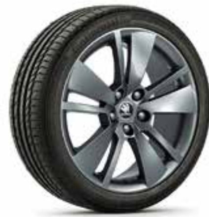
Zenith light-alloy wheel 8.0J x 18" for 235/45 R18 tyres ŠKODA Genuine Accessories in anthracite design (3V0 071 498C HA7)
