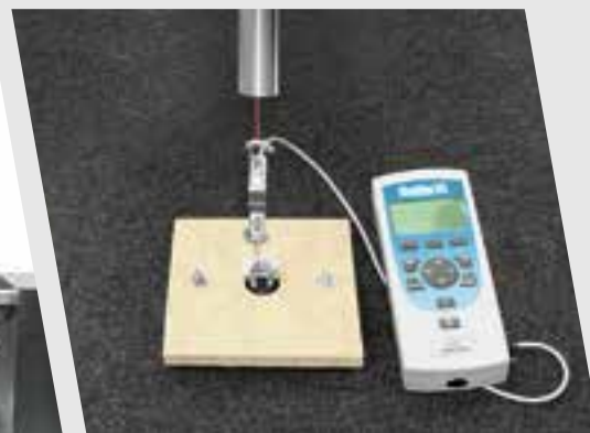
Testing of fixing element strength
