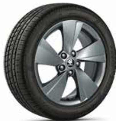
Zeus light-alloy wheel 7,0J x 17" for 215/55 R17 tyres ŠKODA Genuine Accessories in anthracite design (3V0 071 497A HA7)
