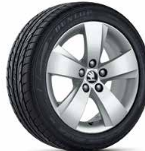
Mato light-alloy wheel 6.0J x 15" for 185/60 R15 tyres in silver design (6V0 071 495 8Z8)
