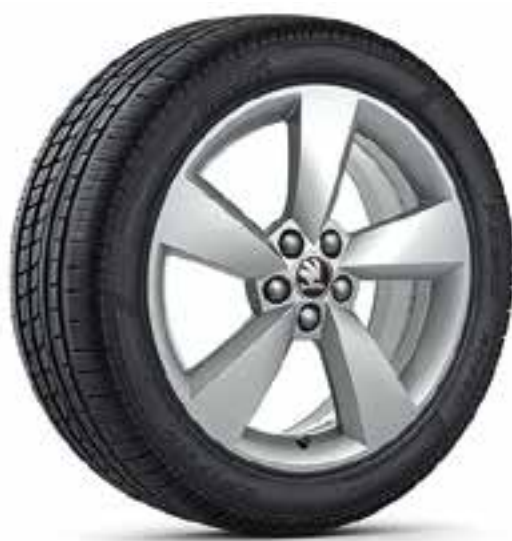
Camelot light-alloy wheel 7.0J x 17" for 215/40 R17 tyres in silver design (5JA 071 497A 8Z8)
