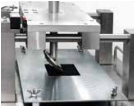
Device for high-heel test Fixing elements strenght testing
