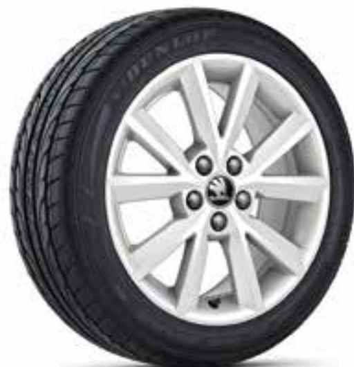
Beam light-alloy wheel 7.0J x 16" for 215/45 R16 tyres in white design (5JA 071 496 FM9)
