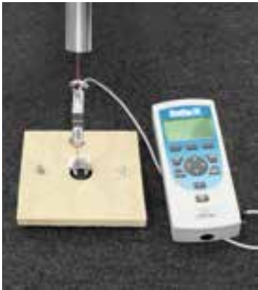
Device for high-heel test Fixing elements strenght testing
