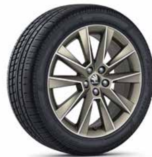
Savio light-alloy wheel 7.0J x 17" for 215/40 R17 tyres in matte platinum design, brushed (5JA 071 497 HZ9)
